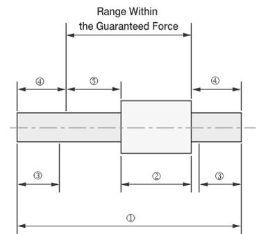
Note: ③ Range outside the guaranteed force: If any part of the moving coil is located within this range, characteristics indicated in *Force and Speed Characteristics* on page 184 cannot be satisfied.
