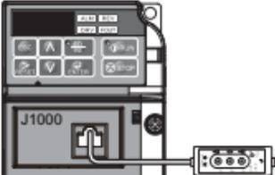
A technical diagram of the J1000 unit. The unit is a rectangular device with a control panel at the top featuring a small LCD screen and several buttons labeled with symbols like 'A', 'V', and 'E'. Below the control panel, the model number 'J1000' is printed. On the right side of the unit, there is an RJ-45 port. A cable is connected to this port and leads to a separate rectangular module with a multi-pin connector, representing the RS232C interface connected to a drive. |
