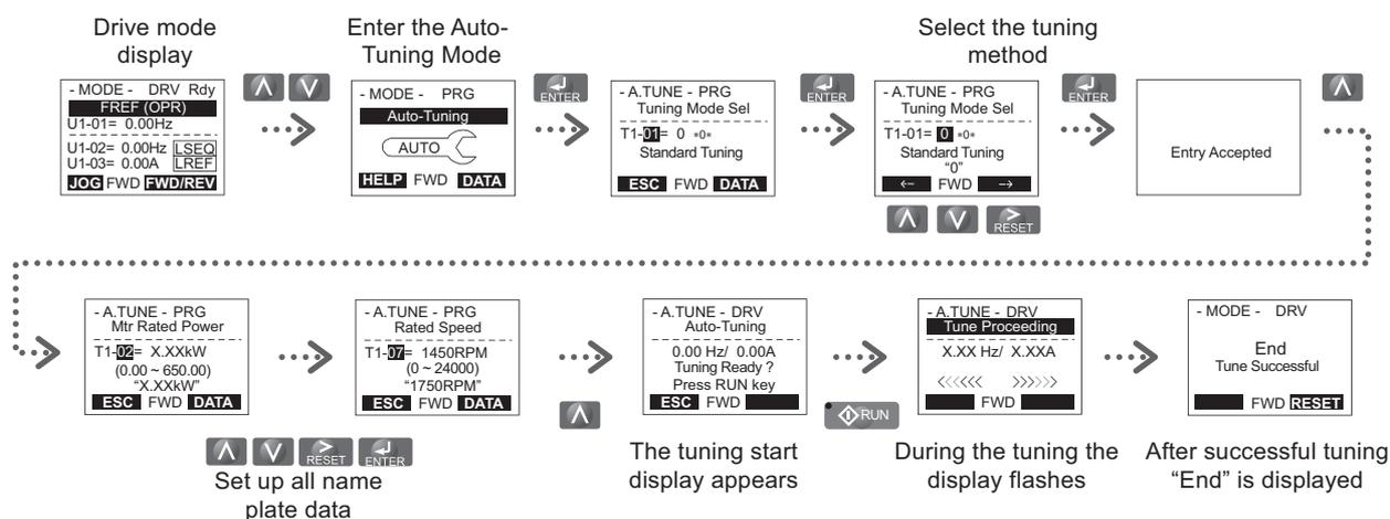
If Auto-Tuning can not be performed for some reason (no-load operation impossible etc.), then set up the maximum frequency and voltage in the E1-□□ parameters and enter the motor data manually into the E2-□□ parameters.
